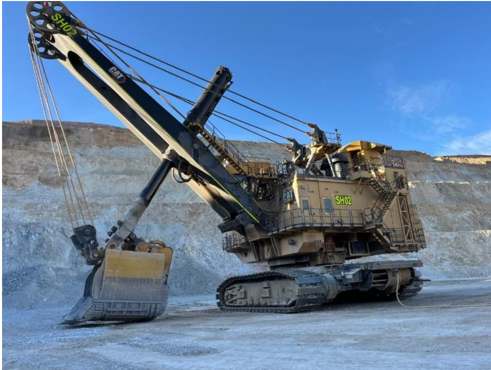
Caterpillar 7495 Electric Rope Shovel
