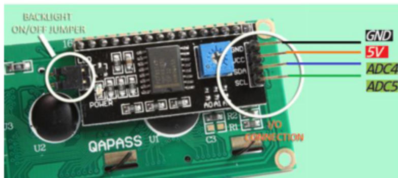
LCD display to Arduino wiring.
