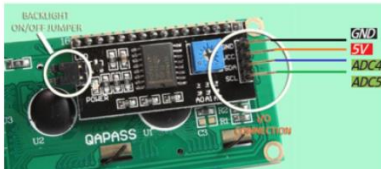
LCD display to Arduino wiring.
